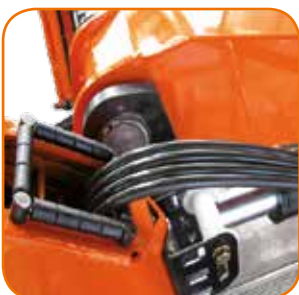
Internal hose routing, good protection for hoses.
